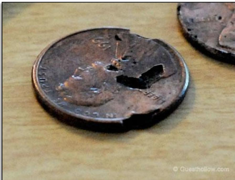
🧐 Did you know that pennies after 1982 are actually zinc coated with copper? We could really see this when we took some of the newer pennies out and observed the partially-dissolved, thin copper coating over a darker metal underneath. Copper is so expensive now that it would cost MORE than a penny for each penny to be pure (actually 95%) copper!
